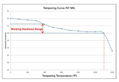
With its high hardness, S7 MQ<sup>®</sup> has excellent resistance and increases lifespan of tools.
